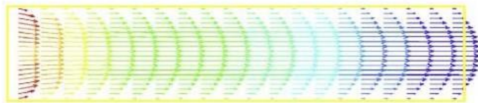
Figure 1.23 Velocity vectors showing the flow development along the parallel-plate channel for Case of flow between two stationary parallel plates
